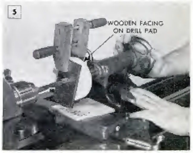
In live drilling, pictured in the photos above and below, the drill usually is held in a geared chuck and driven by the lathe headstock. Flat work is supported by a pad as in the lower views. Note wooden facing
